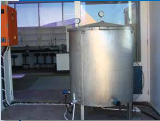
Newly developed steam pot for sterilizing mushroom culture medium.
